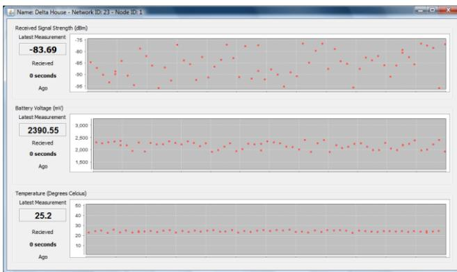
Fig. 3. Screen shot from the monitor and control station PC
