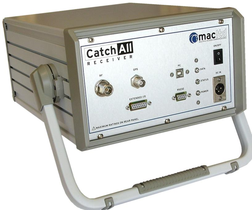
Depending upon the mode of operation, this band can be scanned up to 200 times per second, and with this scanning rate the CatchAll receiver can accommodate an effective scan list size of 200 TETRA or 400 Tetrapol carriers, thereby eliminating the need to carefully design the scan list prior to each measurement run and also removing any requirement to update the scan list during a measurement run.
